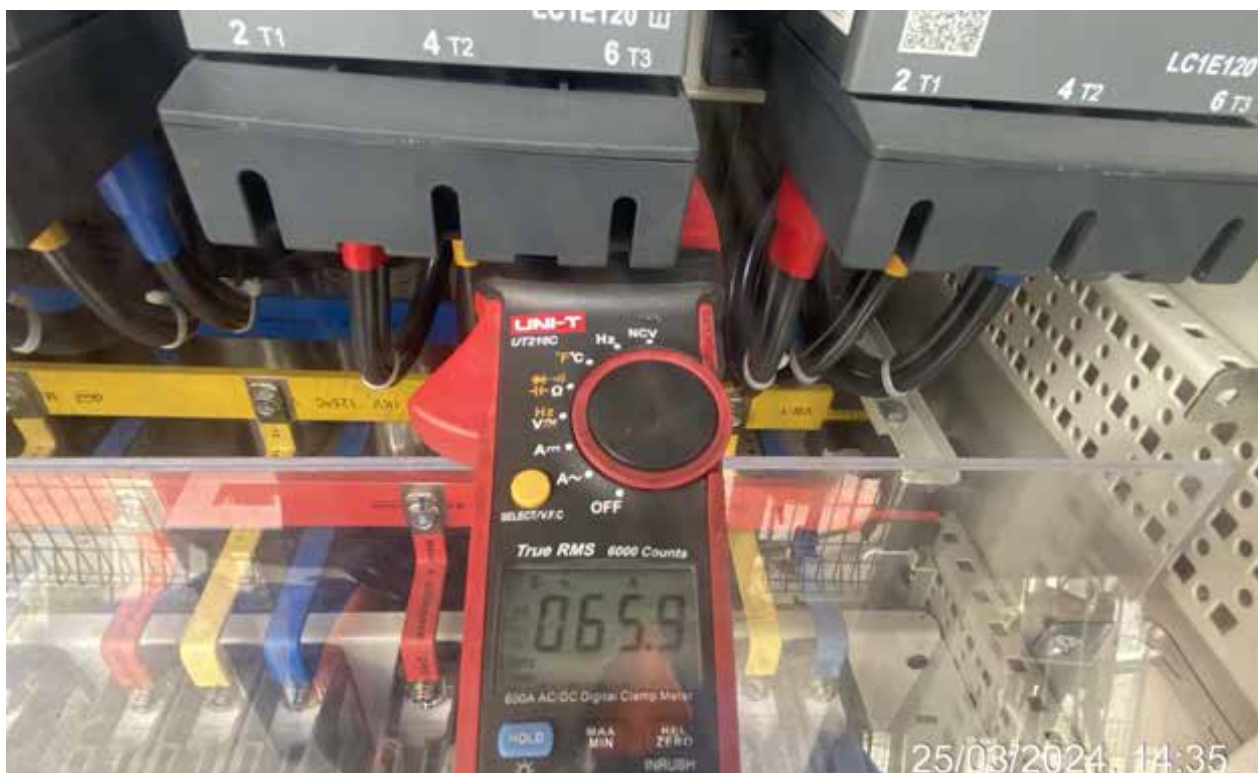
Figure 50: Using a clamp meter to measure current
