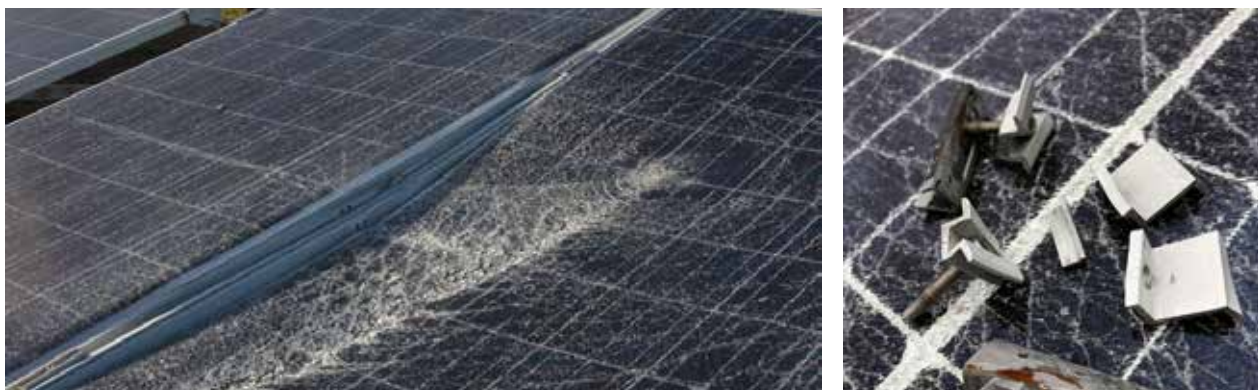
Figure 59: PV panels were cracked and clamps were broken after a storm
