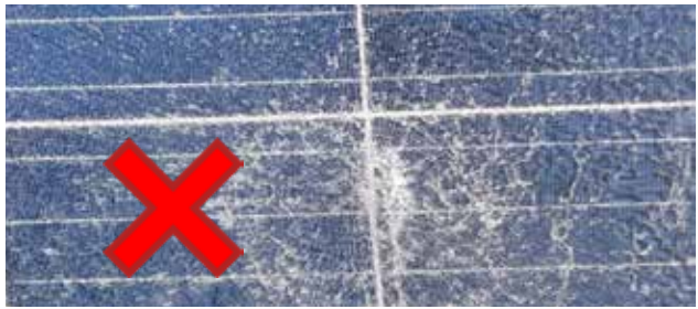
Figure 30: Do not clean damaged PV panels
