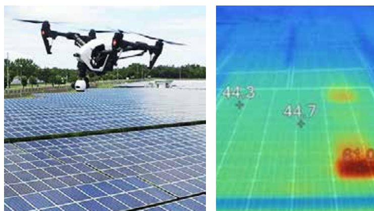
Figure 34. Detecting faults in PV panels using drone with thermal sensors
