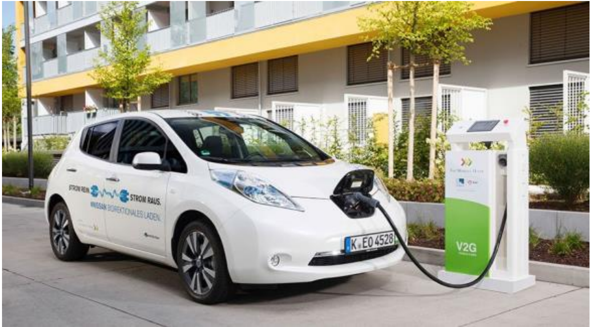
Figure 14: Electric vehicle with bidirectional charging capability (V2G). In aggregation they are used to offer operating reserves [21]
