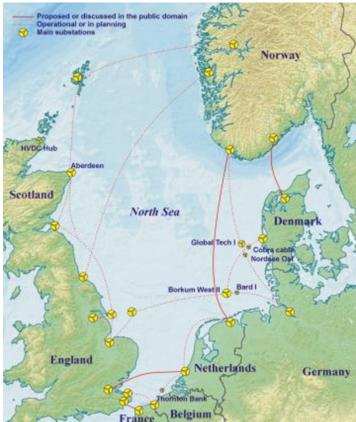
Figure 5: Proposed and operational HVDC links in the North Sea, connecting offshore wind power plants and interconnecting European countries [12]
