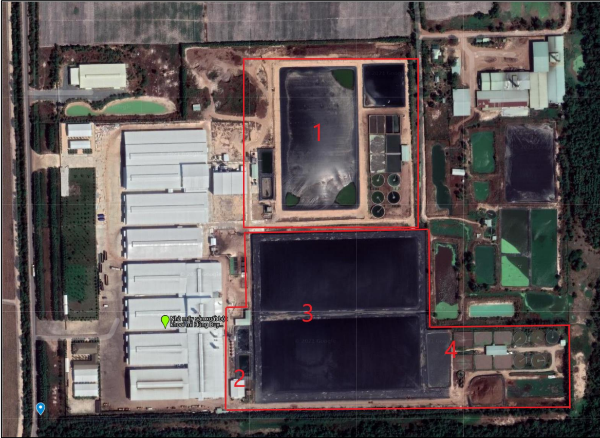
Figure 33: Duy hung cassava factory (google maps) 29 1= wastewater treatment system of new investment in producing modified starch, 2 = wastewater collect tank 3 = two parallel biogas plants, 4 = biogas plant effluent treatment (settlement tank, anoxic tanks, anaerobic treatment and sterilization tanks)
